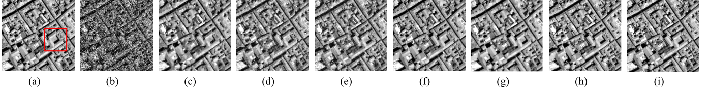
Fig. 5. Pavia city center image before and after denoising. (a) Original image of band 51. (b) Simulated noisy image in Case 2. The restored images of (c) BM4D, (d) TDL, (e) LRMR, (f) LRTV, (g) LSSTV, (h) LLRSSTV, and (i) TV-NLRTD.
